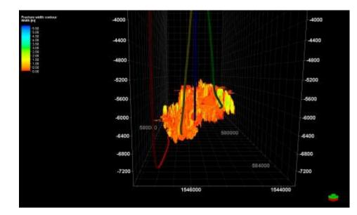
Complex fracture network generation due to the interaction between hydraulic fracture and natural fracture
