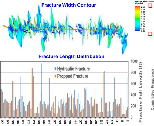
3D non-planar fractures with non-uniform length and height.
