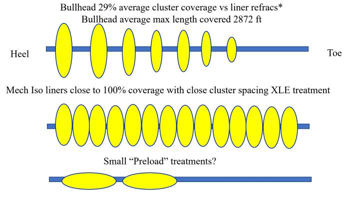
Minimal far field impact expected with small volume preloads only helps primary wells Should have less asymmetric frac protection than larger volume diverted bullheads
