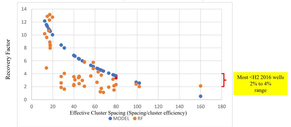
Recovery factors should typically be less than the blue curve, 100% cluster efficiency assumed for curve Abnormally high recovery factors suggest either a bust in the OIP/GIP or production allocation issues
