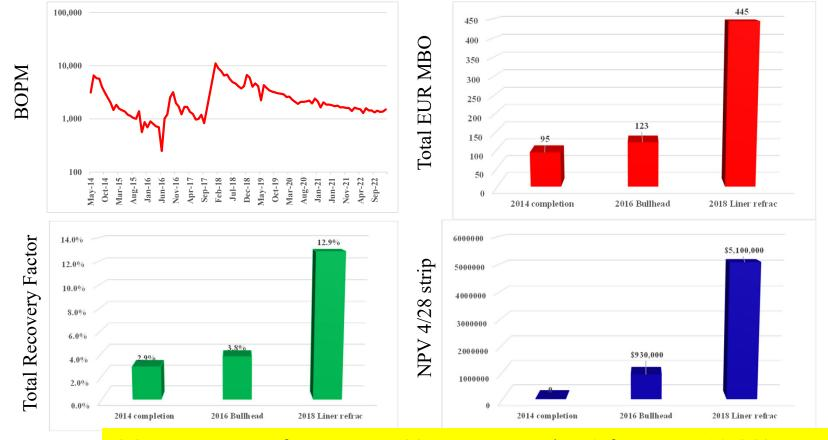
367 MBO post refrac EUR vs 321 MBO actual P50 for EFS, P10 464 MBO Target candidates (excluding parent protection refracs) all above P50 case
