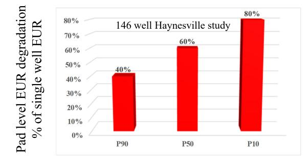
40% estimate made in initial Devon study (Elliott 2019) Assumes only the 1<sup>st</sup> order is damaged for simplified pad level damage estimation SPE 213075 indicates damage beyond first order offset
