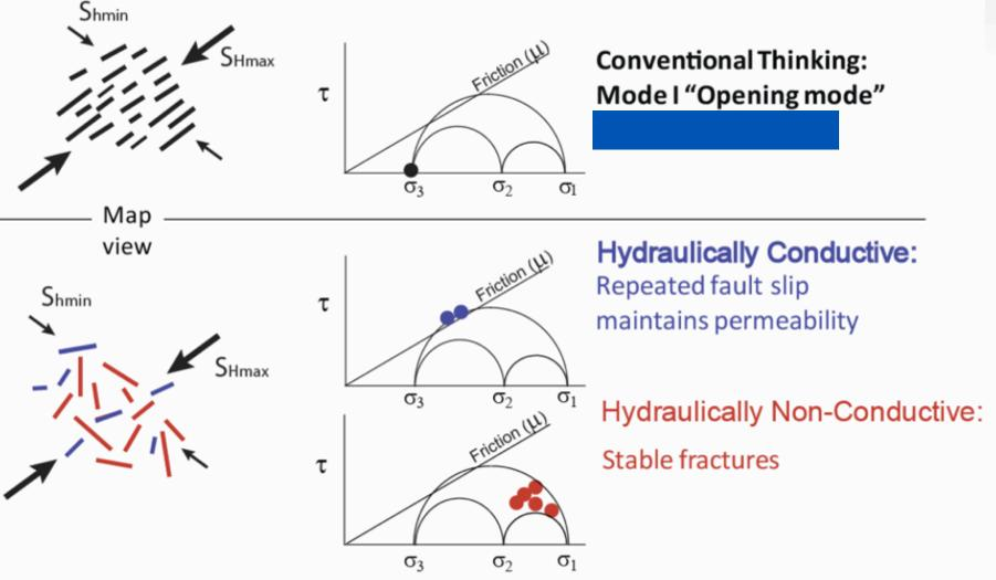
Fractures proximity to frictional failure is highly dependent on the relative stress magnitudes and pore pressures in the reservoir
