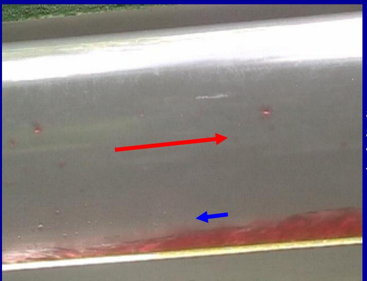
Liquid accumulation at gas velocity less than critical
