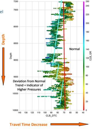
• A pressure gradient can then be derived by using the function of the difference in travel time from the normal compaction and published DFIT data.
