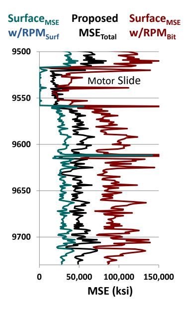
A Surface MSE has historically been calculated when using a motor by multiplying the Surface Torque times either the string speed or bit speed
