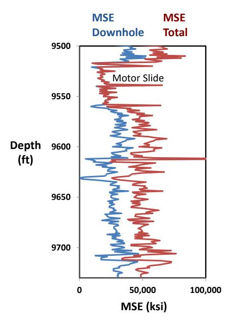
The visual difference between the MSE<sub>Downhole</sub> and MSE<sub>Total</sub> should be the energy being lost in the drill string. This may be a useful diagnostic for loss of weight or torque transfer.
