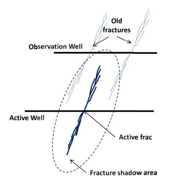
Pressure inside the active extending fracture compresses the fluid in the passive fractures in the adjacent shut-in passive monitor well There is no direct fluid migration between the fractures
