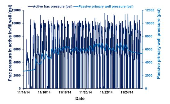
Daneshy Consultants International Frac-driven pressure build-up in the shut-in offset well caused extension of its existing fractures
