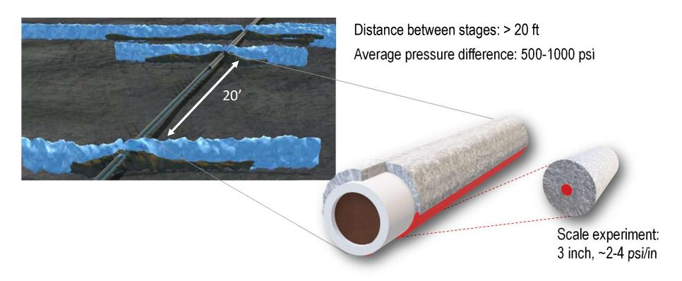
Mud channel laboratory model with well-controlled parameters
