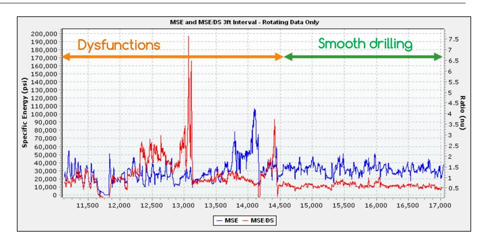
Significant dysfunction in a few places, MSE spikes and frequently changing ratio. Efficient, steady state drilling with low to no dysfunction. Ratio constant around 0.5
