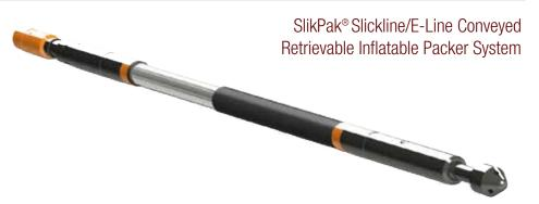
SlikPak is a battery-powered assembly that can run 2.13 in. to 14.5 in. inflatable bridge plugs or packers. The inflation fluid can be obtained from the wellbore or carried in adaptable fluid chambers. SlikPak is ideal for remote locations or wellsites with a small footprint.
