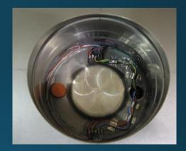
Strain pocket, gages attached to wall
