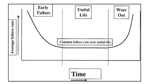
Assumption on exponential distribution can be tested in Survival Probability plot with statistical distribution curve fit and Weibull parameter estimation.
