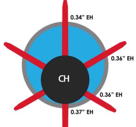
**CH Perforator** charge in 3.125" 6spf 60° gun in 5.5" 23# P-110
