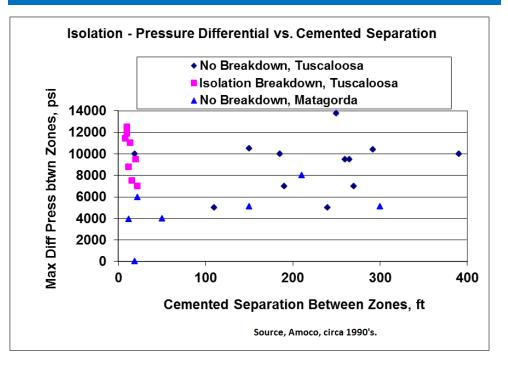
SPE 166142, Barrier vs. Well Failure, King
