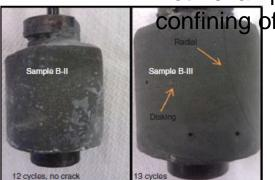
Fig. 9—The 13th cycle, the failure cycle under 2,000-psi differential.
