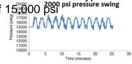
Fig. 10—HP/HT cement-sheath cyclical-loading test, 12 cycles of a 2,000-psi magnitude, Set B.
