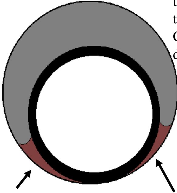
Area of undisplaced mud – a mud channel remains, requiring squeezing.
