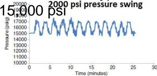
Fig. 10—HP/HT cement-sheath cyclical-loading test, 12 cycles of a 2,000-psi magnitude, Set B.
