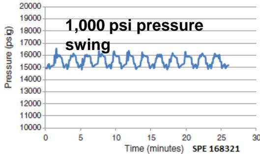
Fig. 6—HP/HT cement-sheath cyclical-loading test, 12 cycles of a 1,000-psi magnitude, Set A.
